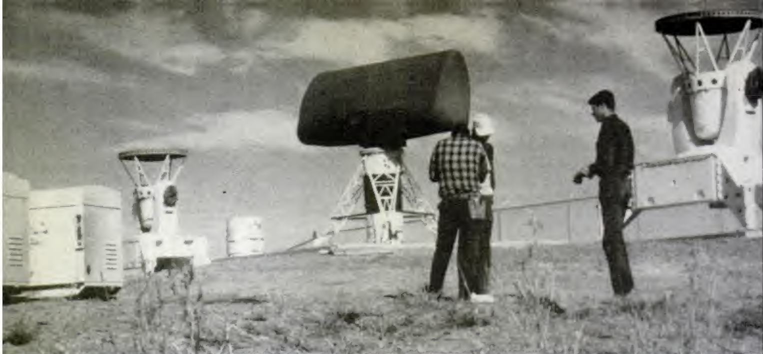
RADAR INSTALLATION IN COLORADO is used to track high-flying balloons for wind computations and to scan for precipitation echoes. Work is part of research involving the seeding of wintertime snow clouds
